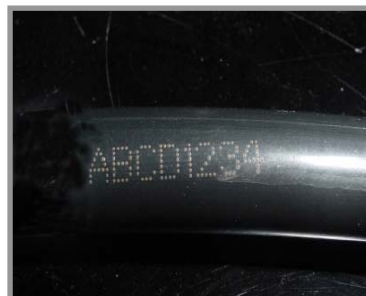
Marking PVC cable
